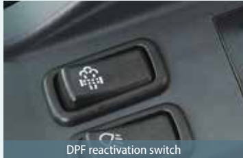
DPF reactivation switch If the monitor warning goes off, the filter should be reactivated manually using a switch.
