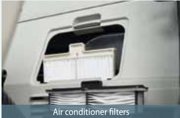
Air conditioner filters Internal and external air conditioner filters can be easily removed without tools for cleaning.
