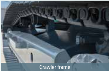
Crawler frame Special crawler frame design is easily cleaned of mud.
