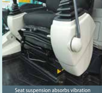
Seat suspension absorbs vibration
